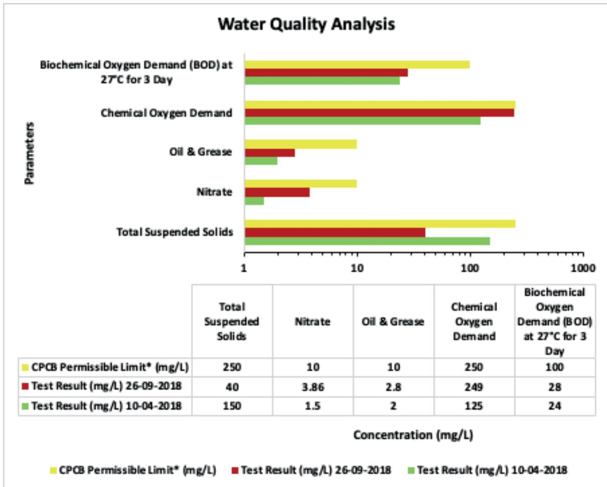
Figure: Water quality analysis of the effluents from the disposal tank
